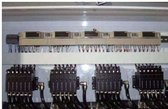
Flexible automation – Four, six station manifolds control an End-of-Arm Tool that configures different zones of cups to handle a wide variety of stamped metal parts. No tool change required.
