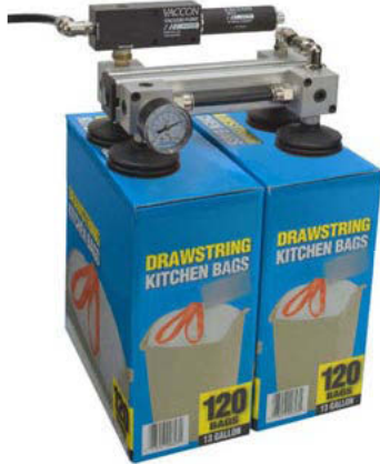
VP80-200M transfers boxes for palletizing operation
