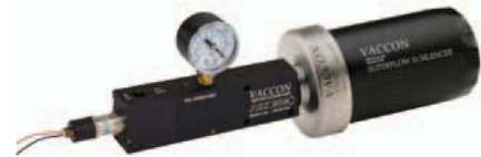
Specifications: VP80BV-200H with FA51-3/8 optional silencer and VG-150 vacuum gauge. Weight: 1 lb 9 oz [707.6g] Noise Level: 72dB
