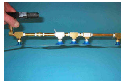
Received customer samples at 8 am, emailed photo of VP10 pump with flat cleated cups handling pliable plastic strips by 9 am – packaging application.
