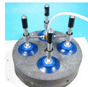
VDF pumps with flat cleated cups handle 42 lb graphite spacer for nuclear industry.
