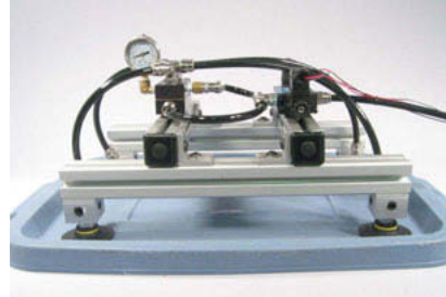
Vaccon EDAT with Multi-port pumps, manifold blocks and flat cleated cups – pick and place plastic lids for packaging application.
